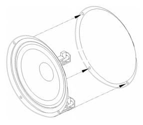
**STEP D.** Carefully tighten the dog-ear screws until the frame is flush with the wall. For the in-wall frame, start with the center dog-ear clamps. Then use a level to correctly align the speaker and then tighten the remaining dog-ear clamps. For the in-ceiling frame, start with one dog-ear clamp and then tighten the dog-ear clamp on the opposite end. Do not excessively tighten the dog-ear clamps. Doing so will cause damage to the wall and speaker frame.
